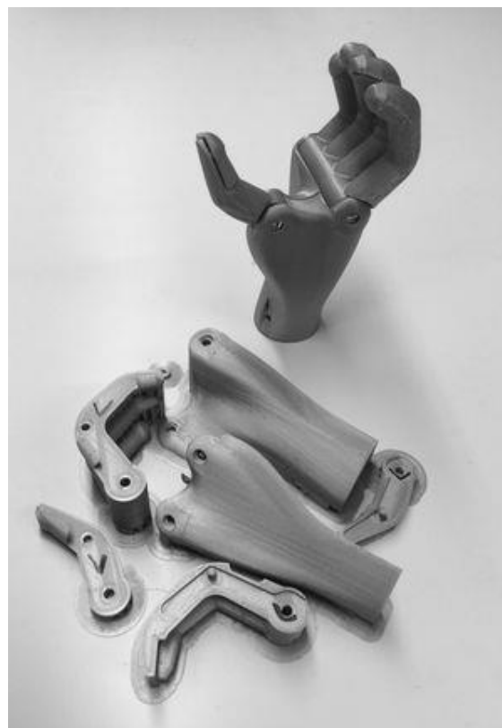
Figure 1. The 'Hundred Dollar Hand', printed parts and assembled.
