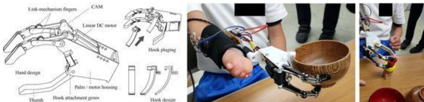
Figure 1. Design of the prosthetic hand, and screenshots from the pilot test.
