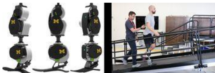
Figure 1. (Left) Rendering of the OSL. (Right) Patient walking up a ramp using the OSL.
